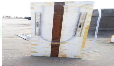
Figure 4.11: pictorial view of U-tube manometer
