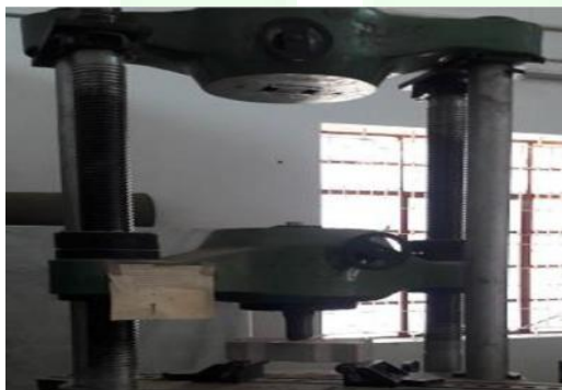
Fig 9 Flexural strength test conducted by using Universal Testing Machine
