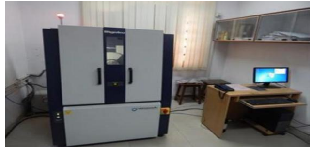
Fig 10 Multipurpose X-ray diffraction system (Rigaku ULTIMA IV).
