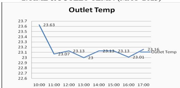
Fig. No. 5.6 Variation of Outlet temperature with time
