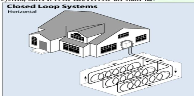
Fig No.1.1 :Earth tube Heat Exchanger (Closed Loop System)
