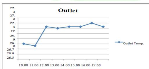
Fig. No. 5.2 Variation of Outlet temperature with time
