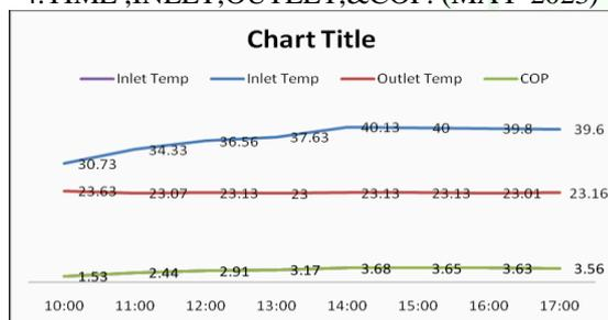
Fig. No. 5.8 Variation of Inlet, Outlet Temp. & COP with Time
