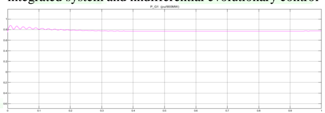
Fig. 27: Power stability in p.u at the generating terminal of machines in case 2
