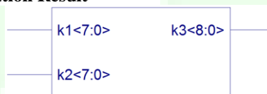
Figure 4 View Technology Schematic of 8-bit Kogge Stone Adder
